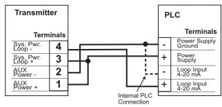
Example: Two transmitters connected to PLC/Recorder
